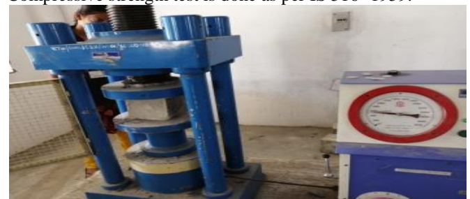
Fig 1: Testing of Compressive strength for concrete
