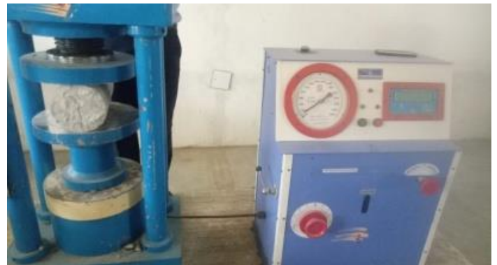
Fig 2: Split Tensile strength Test
