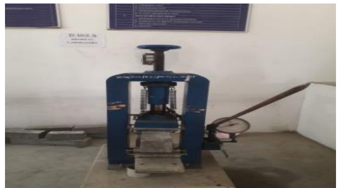
Fig 3: Testing of Flexural strength for concrete
